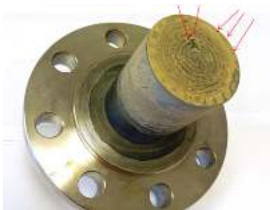
Figure 3 & 4: Within one year the Tantalum diaphragm is severely damaged due to loss of corrosion resistance due to welding.
