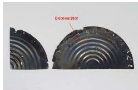
Figure 3 & 4: Within one year the Tantalum diaphragm is severely damaged due to loss of corrosion resistance due to welding.
