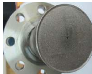
Figure 1: Hastelloy C276 diaphragm disappeared within one-year operation
