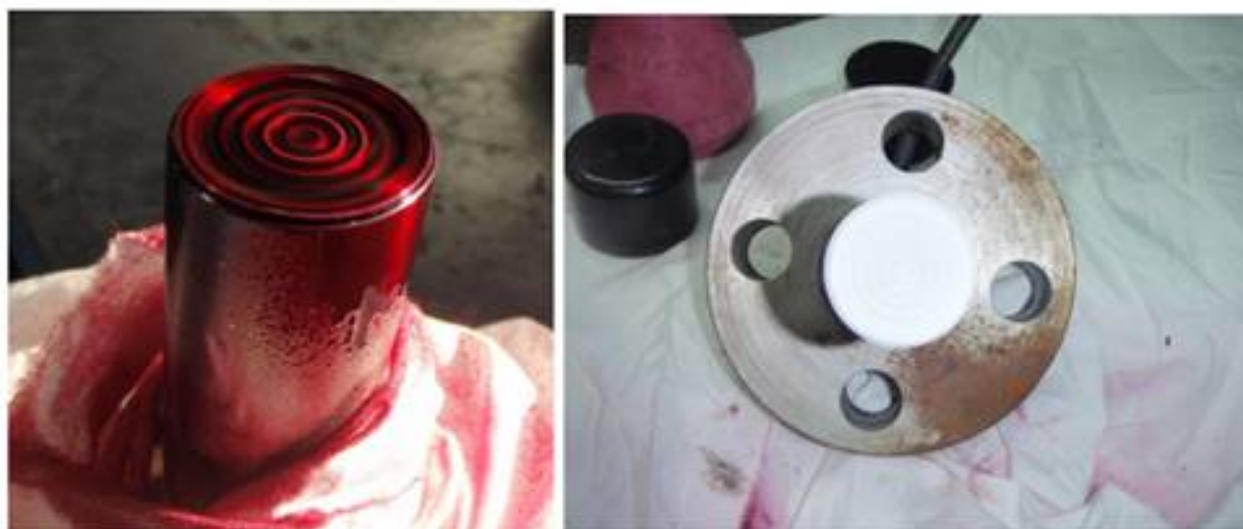
Dye penetrant test of diaphragms
