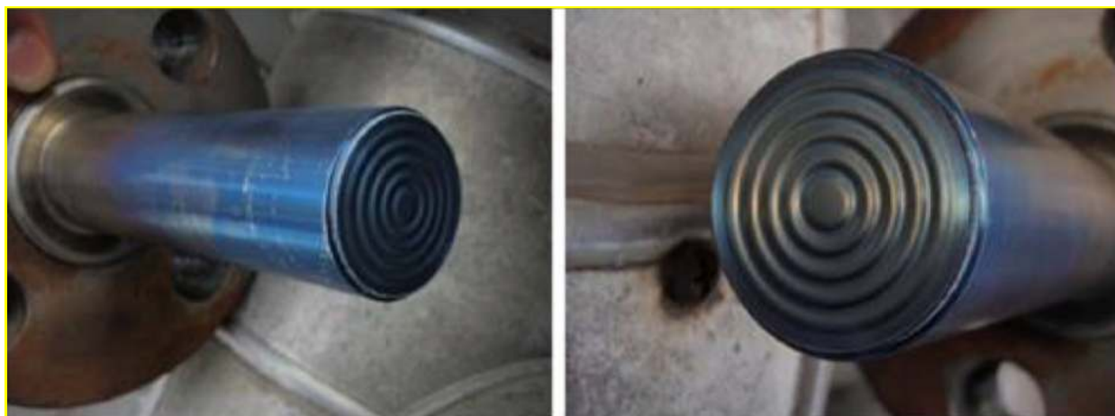
Blue colors as a result of passive corrosion
