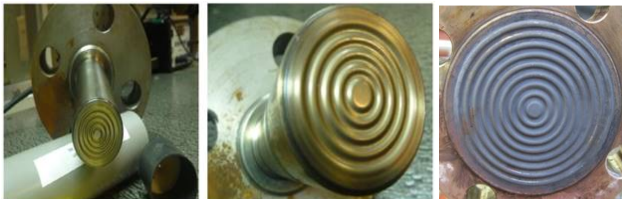
See above examples of a diaphragm with dents. Second picture is a typical example of a bulged diaphragm
