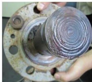
Picture 2: Corrosion damage SS 316L
