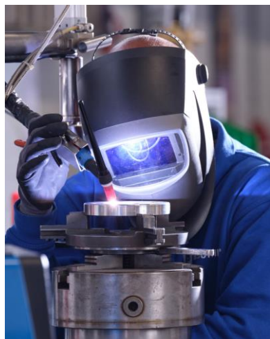
Picture 9: Badotherm welder welding the Safurex® diaphragm
