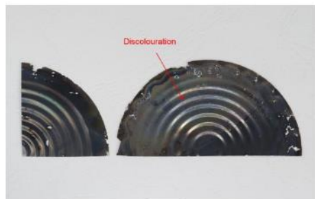
Picture 1: Corrosion damage HAZ Tantalum
