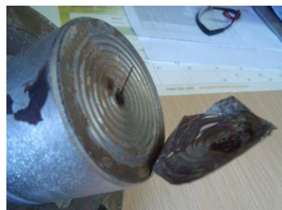
Picture 3: Weld damage Zirconium
