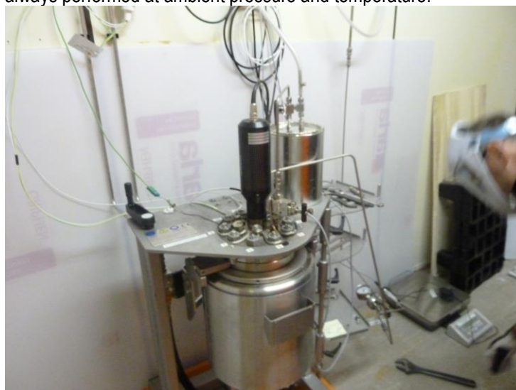
Picture 10: Autoclave used for the HP experiments
