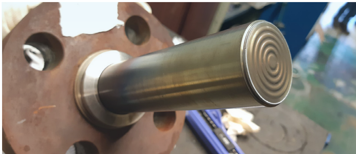
Picture of Badotherm's zirconium diaphragm seal system taken during 2021 turnaround. Diaphragm seal body and diaphragm are slightly discolored, but without any sign of mechanical damage or active corrosion. Still in perfect shape after 3 years in operation
