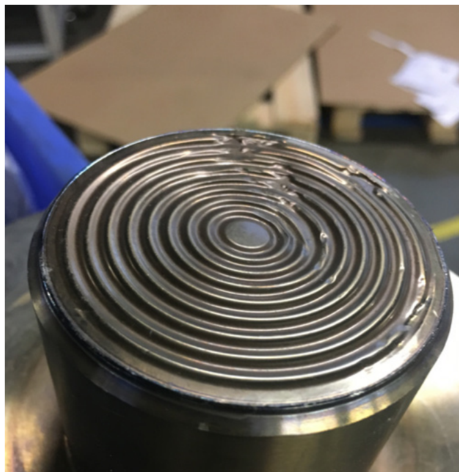
Examples of Badotherm diaphragm seals that were damaged as a result of wrong handling during the turnaround and the use of power jet cleaners during the 2018 plant stop.
