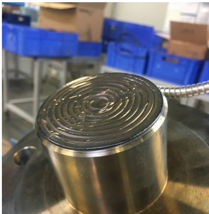
Examples of Badotherm diaphragm seals that were damaged as a result of wrong handling during the turnaround and the use of power jet cleaners during the 2018 plant stop.
